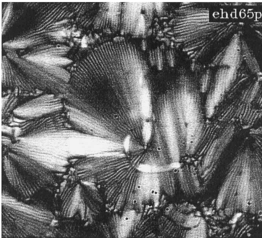
Figure 15. Electrohydrodynamic instability in m7tac racemate at T=125^{\circ}\text{C} , f=1\text{ Hz} and V=65\text{ V} . The rolls are locally parallel to the layer normal.
